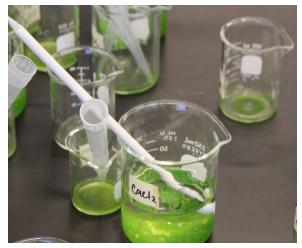
Alginate "beads" containing microagle suspended in gel, used to treat wastewater
