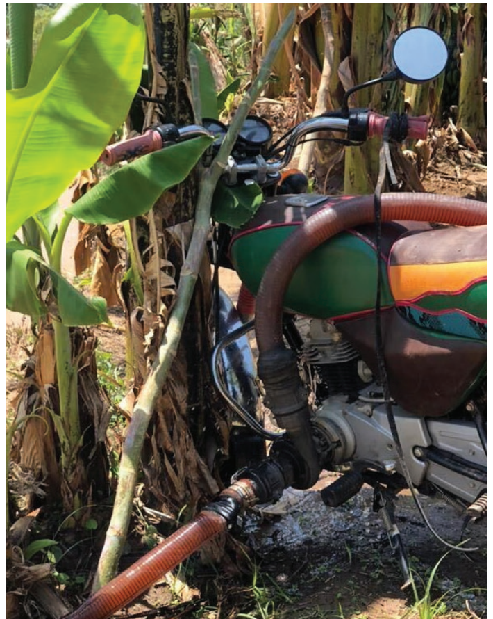
Photo showing the Agriworks mobile, motorbike-powered water pump.
