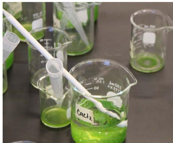
*Alginate "beads" containing microalgae suspended in gel, used to treat wastewater*
