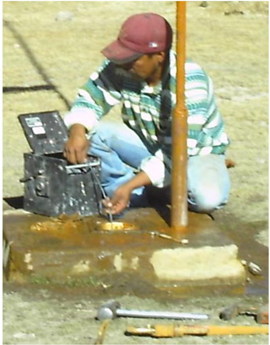
SWL measurement with electric probe.
