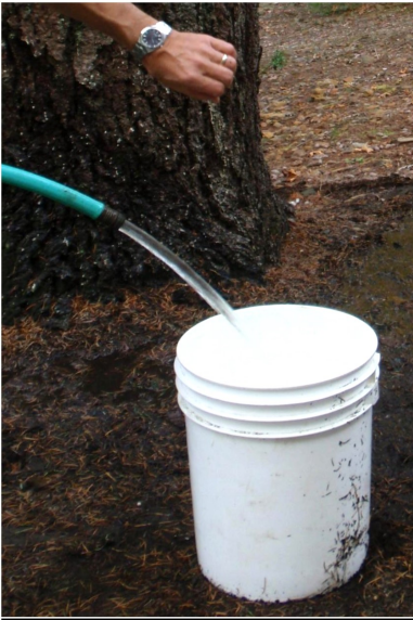
Bucket timing flow from a domestic well
