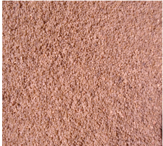
A sample of filter pack material
