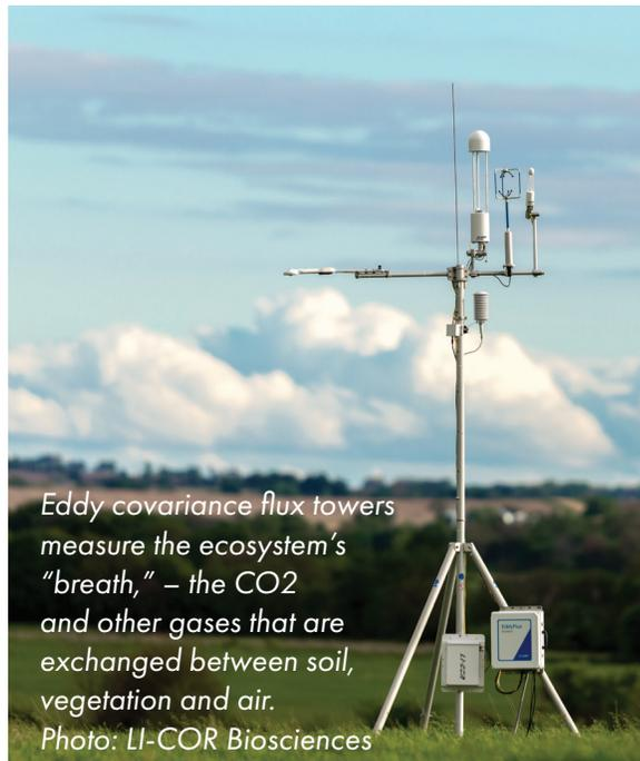
*Eddy covariance flux towers measure the ecosystem's "breath," – the CO<sub>2</sub> and other gases that are exchanged between soil, vegetation and air.*
