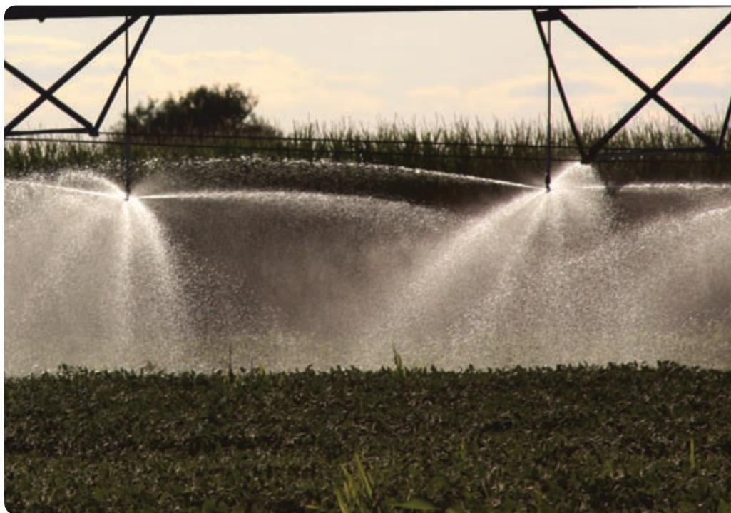
Center pivot with low-pressure spray nozzles and hose drops
